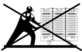
Move the transformer, whether alone or enclosed in an integral sheet metal box, by leverage against lower clamps or by means of its towing holes only.
